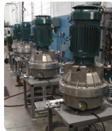
Seal Validation Program With Multiple Test Rigs
