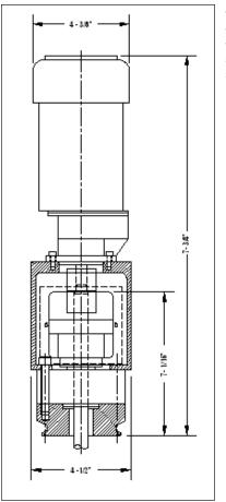
This configuration shows the standard single seal; the image on the front shows the optional double seal unit.
