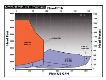
Sundyne debuted its first high-head, low-flow pump nearly 50 years ago, and the competition has been playing catch up ever since. The LMV/BMP 341 is available in a heavy duty single stage configuration, featuring a compact footprint and the rugged reliability we've built our reputation on.
